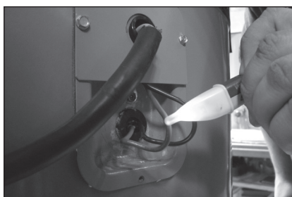
Figure 43 - Non-Contact Circuit Tester.
