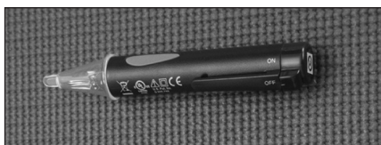
Figure 39 - Non-Contact Circuit Tester.
