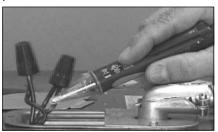
Figure 37 - Non-Contact Circuit Tester
