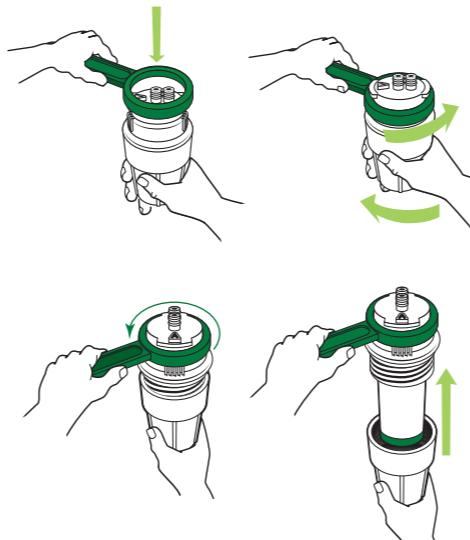
Do not use tools other than undercounter wrench to remove or tighten sumps. Over tightening can cause damage and result in leaking.
