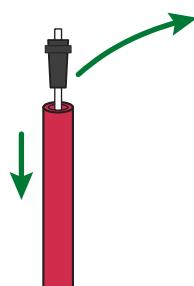
**3** Remove the membrane cartridge from the system by rotating the sump to the left and pulling down.
